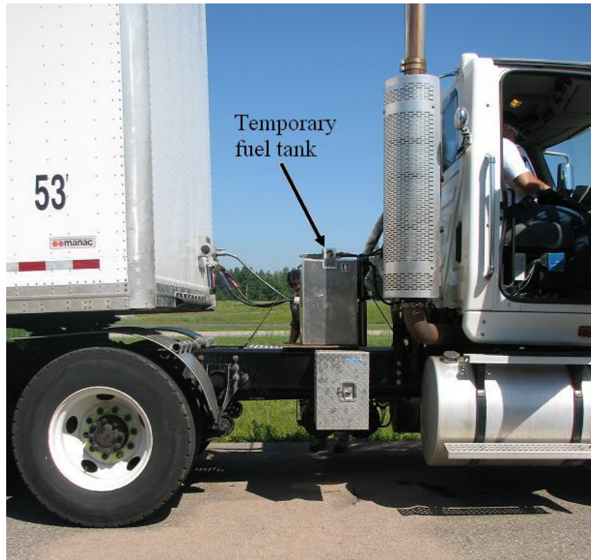
Figure 4. Installation of the temporary fuel tanks.
