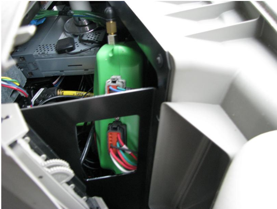
Figure 5. FMZ Device installed on the test vehicle.
